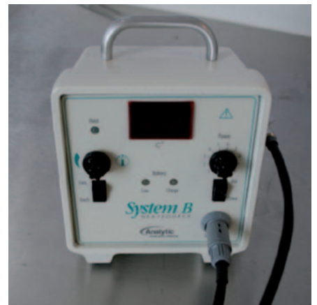
Fig. 23 System B (SybronEndo): capable of reaching temperatures in excess of 600 °C
